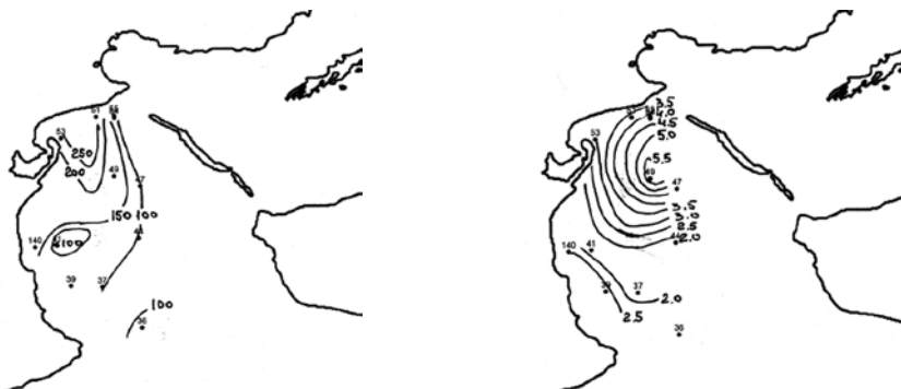
Fig. 6.2.8b. Real and aluminum normalized TPHs distribution in the Kerch Strait bottom sediments on 8 July 2009.
