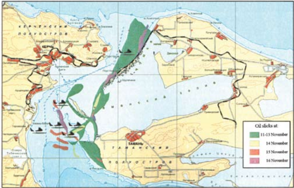
Fig. 8.4c. Scheme of oil expansion resulting from the 11 November 2007 oil spill accident in line with results of the Kerch Strait aerial survey conducted on 11–16 November 2007 (Matishov G. G., 2008). Periods: in green — 11–13 November, in yellow — 14 November, in red — 15 November and in pink — 16 November.
